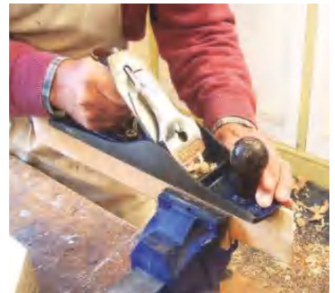
▶ Pic.9 Planing the bottom edge of the sides
